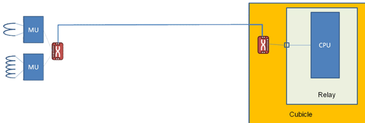
Figure 6 IEC 61850 Merging Unit based sensor and IED
