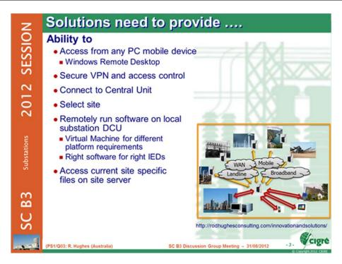
Once logged in to the Central Distributed Control Unit (as for example the DCU provided by 7com Ltd and distributed Rod Hughes Consulting Pty Ltd), this can provide the operator through Windows Remote Desktop (\*avoiding need for any special software on their PC) selection and access to the remote site through secure VPN by any variety of communication networks- including Mobile 3G in order to retain segregated or alternative comms to the corporate WAN.
